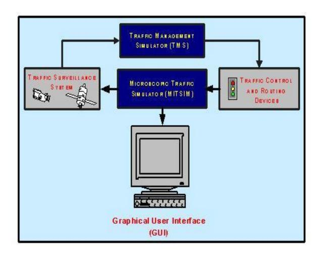
Figure 4-1: Components of MITSIM and their interactions
