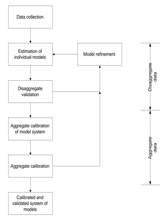
Figure 1-1: Calibration Framework
